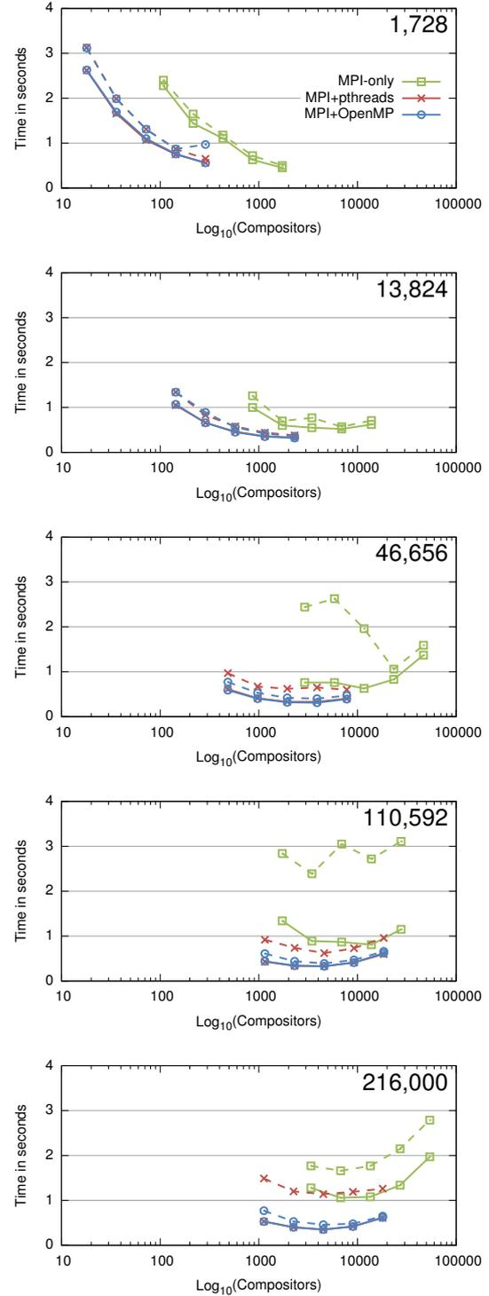
**Figure 7:** Compositing times for different ratios of compositing PEs to total PEs. Solid lines show minimum times taken over ten trials each for two different views; dashed lines show the corresponding mean times.
