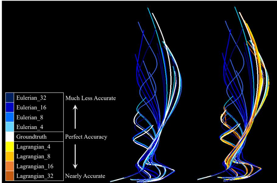
Figure 9. Pathline visualizations to compare the accuracy of pathlines traced using two methods: Eulerian and Lagrangian. Lagrangian\_ $X$  and Eulerian\_ $X$  denote configurations that store data every  $X^{th}$  cycle, i.e., the size of the interval. Left: five ground truth pathlines and the corresponding Eulerian pathlines. Right: five ground truth pathlines, and the corresponding Eulerian and Lagrangian pathlines.
