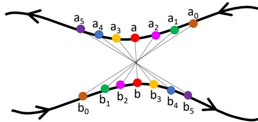
*Figure 50.* The figure shows the pairs of points in a spatial window used by Chen et al. [92]. The pairing considers velocity direction along the streamline and thus measures shape and orientation similarity.
