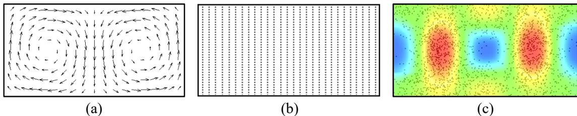
*Figure 4.* An illustration of two possibilities for seed placement given the Double Gyre vector field. Figure (a) shows a vector glyph visualization. Figure (b) presents a simple uniform seed placement and Figure (c) colormaps an entropy field derived from the vector field and shows seed placement with a density proportional to the value of entropy.
