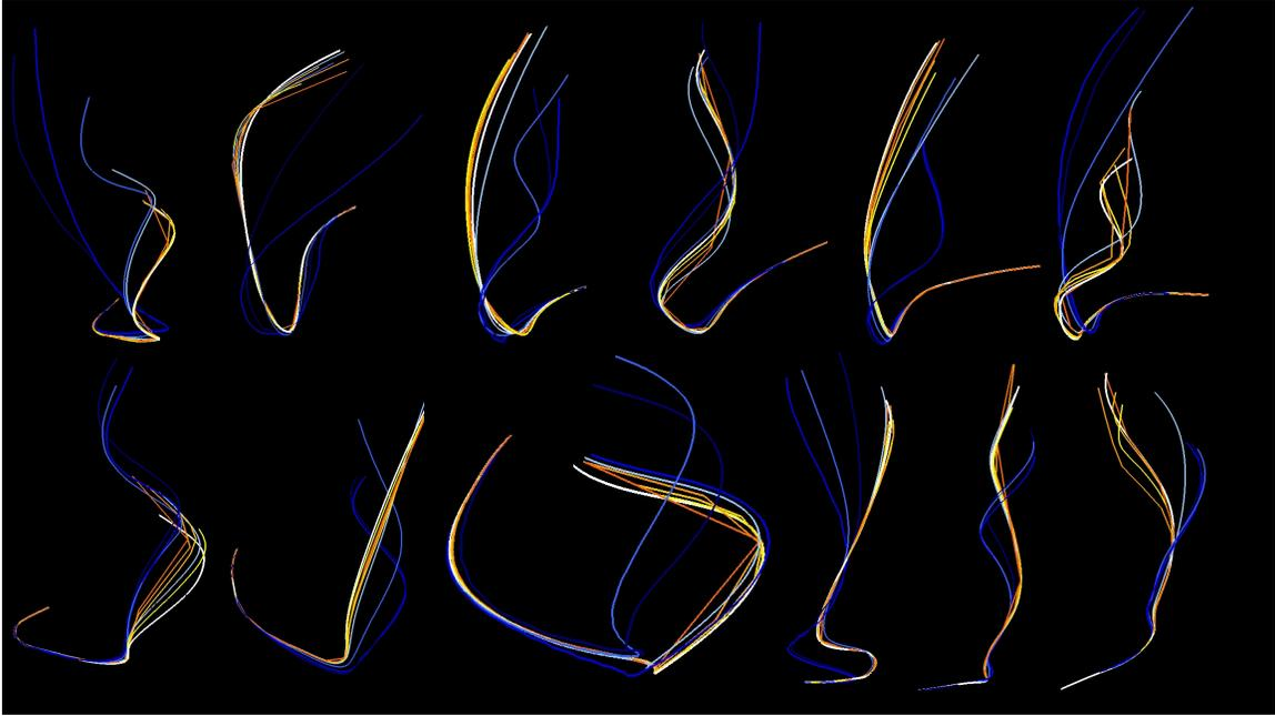
*Figure 10.* Twelve sets of pathlines traced using multiple Eulerian and Lagrangian configurations. Each set shows a ground truth pathline, and four Eulerian and Lagrangian pathlines each. The color scheme is the same as that described in Figure 9. Overall, Lagrangian pathlines more closely follow their respective ground truth trajectories and the Eulerian pathlines are less accurate in settings of temporal sparsity, i.e, configurations with large intervals between saving data to disk.
