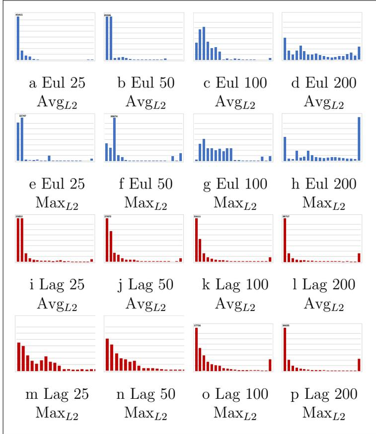
Figure 44. **Nyx** experiment histograms for 50,000 test particle interpolation errors. Each plot has 20 bins, ranging from 0 to  $>0.44$ , with bar height encoding number of particles. Horizontal grid lines mark increments of 2,000.
