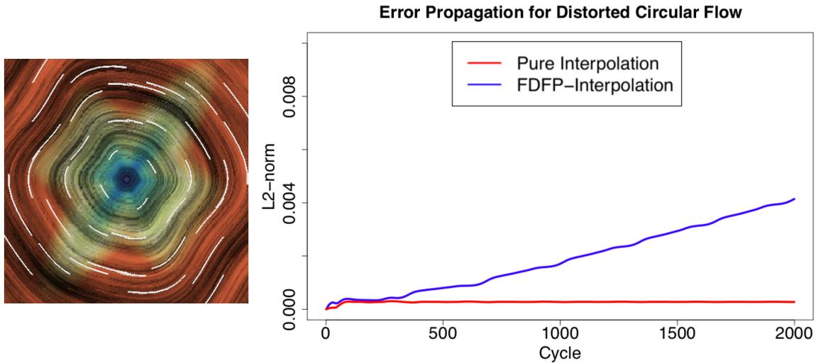
*Figure 16.* Motivating result comparing FDFP-Interpolation to pure interpolation on an analytic data set of distorted circular flow data. The image on the left is the LIC of the flow field (color encodes the velocity magnitude). The white lines are the FDFP basis trajectories. The image on the right is a plot of error propagation over 2000 cycles. In contrast to FDFP-Interpolation, the pure interpolation only shows local interpolation error and has no error propagation.
