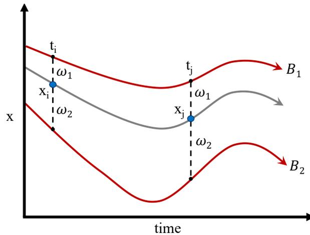
*Figure 7.* Interpolation of a new particle trajectory (gray) using previously computed basis trajectories ( $B_1$  and  $B_2$  in red). Each position along the new particle trajectory is calculated by following basis trajectories. At time  $t_i$ , weights  $\omega_1$  and  $\omega_2$  are calculated based on the distance of  $B_1$  and  $B_2$  from  $x_i$  respectively. The weights are then used to estimate  $x_j$  at time  $t_j$ . This process can continue to trace the complete trajectory.
