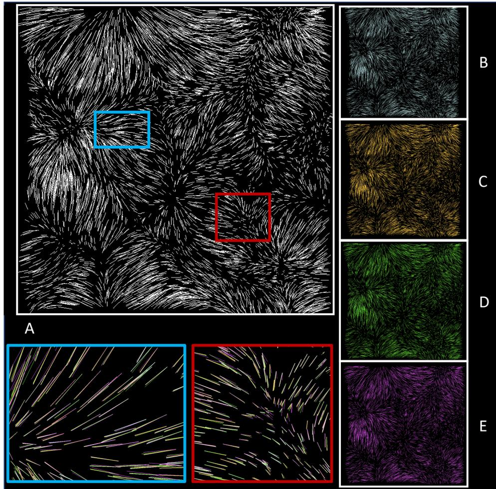
Figure 41. A qualitative comparison of pathline reconstruction over one interval for the Nyx data (**Interval = 25** case). For each configuration we specify **DS-1** and **PHE-1** as (Bytes, Cell Side%). Image A (white) is the ground truth, B (light-blue) is Eulerian (227MB; 2.29%), C (yellow) is Lagrangian 1:1 (232MB; 11.61%), D (green) is Lagrangian 1:8 (27MB; 37.27%), E (pink) is Lagrangian 1:27 (8MB; 72.727%).
