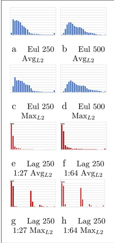
Figure 43. **SW4** experiment histograms for 90,000 test particle interpolation errors. Each plot has 25 bins, Eulerian bins range from  $<0.6$  to  $>15$ , Lagrangian bins range from 0 to  $>0.2$ , with bar height encoding number of particles. Horizontal grid lines mark increments of 2,000.
