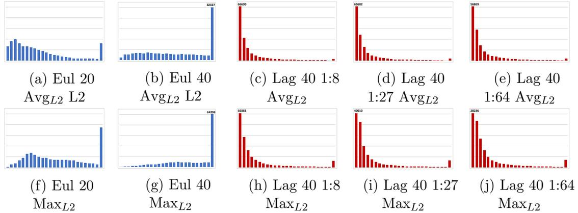
Figure 37. **Cloverleaf3D** experiment histograms for 100,000 test particle interpolation errors. Each plot has 25 bins, ranging from 0 to  $>0.05$ , with bar height encoding number of particles. Horizontal grid lines mark increments of 5,000.
