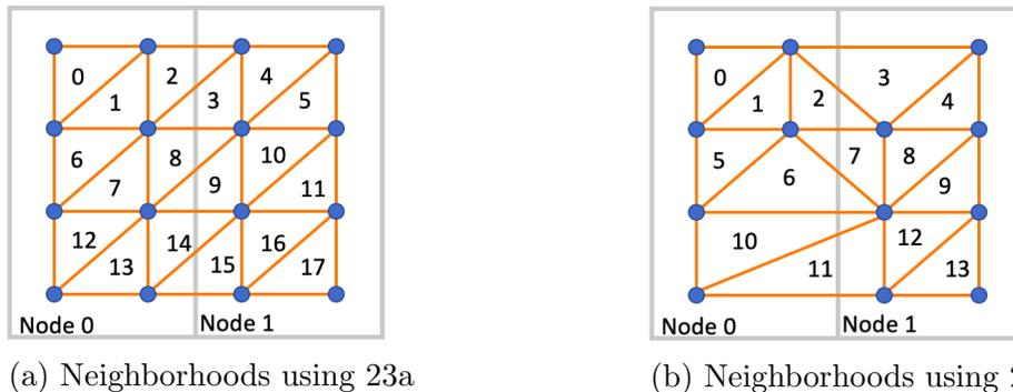
*Figure 24.* Notional examples of neighborhoods produced using triangulation over basis flows shown in Figure 23. The blue circles represent starting locations of basis flows saved to disk.
